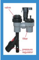
Irrigation valves are designed to work within a certain pressure range (pounds per square inch or psi) and flow range (gallons per minute or GPM). If you redesign your system and use low flow irrigation, the flow through the valve may be so low that your existing valve will not operate effectively and may get stuck in the "open" position, wasting water. If you have flow lower than 5 GPM per valve, check your valve specifications for flow range to determine whether or not to replace your valves.
